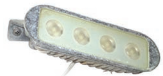
A powder coated aluminium floodlight with housing degradation
