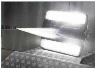
High pressure water & steam jet cleaning
